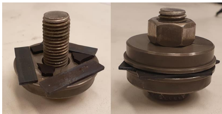
Figure 6. The equipment used to investigate the pressure on the swelling. In the left image, the upper metal plate is off to show how the spacers and the rubber pieces were placed. In the right image, the upper metal plate is on.
