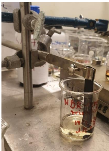
Figure 7. Set-up for the rubber strands. The strand is placed approx. 10 mm down in the beaker without touching the bottom of the beaker.
