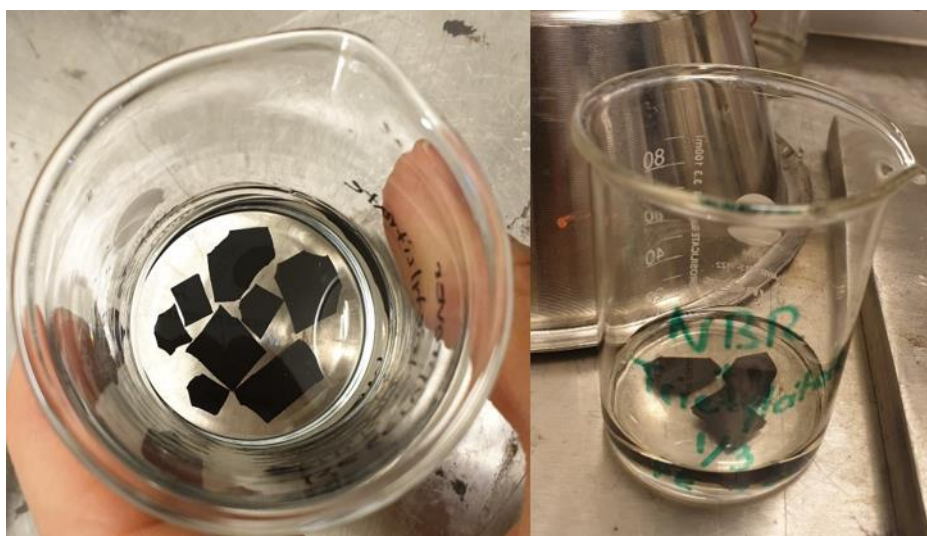
Figure 5. Set-up for the free swelling test. The pieces are cut into different sizes and shapes.
