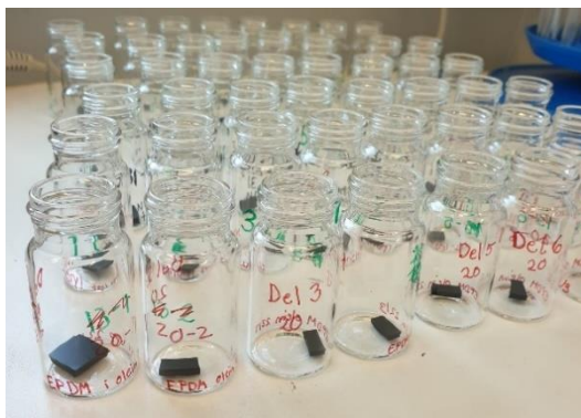
Figure 8. Image of six strands that have been cut to be prepared for extraction.
