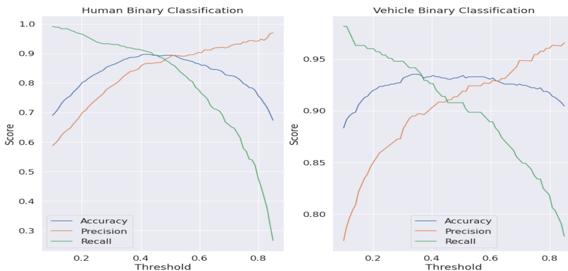
Figure 5.5: Plots illustrating the relationship between classification threshold and various scores of interest when the problem is cast to be one of binary classification where the model employed is based on PCA and KNN. To the left a positive represents a human classification and to the right a positive represents a vehicle. As the classification threshold increases, the precision score continues to improve at the expense of accuracy and recall.
