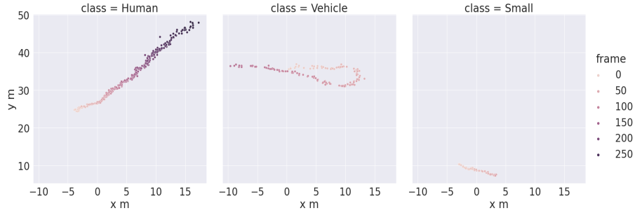
Figure 1.1: Example of point-cloud data tracks for each class. Each point represents the mean value of the x and y coordinates in a given frame. The plot illustrates the fact that Small class tracks tend to be relatively short.
