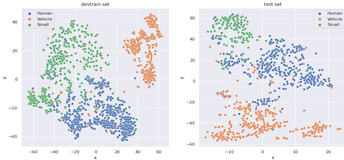
Figure 5.2: t-SNE plot of the observed embeddings on the first 21 frames of each track in the train and test sets of an encoder network fitted with batch size 4096.
