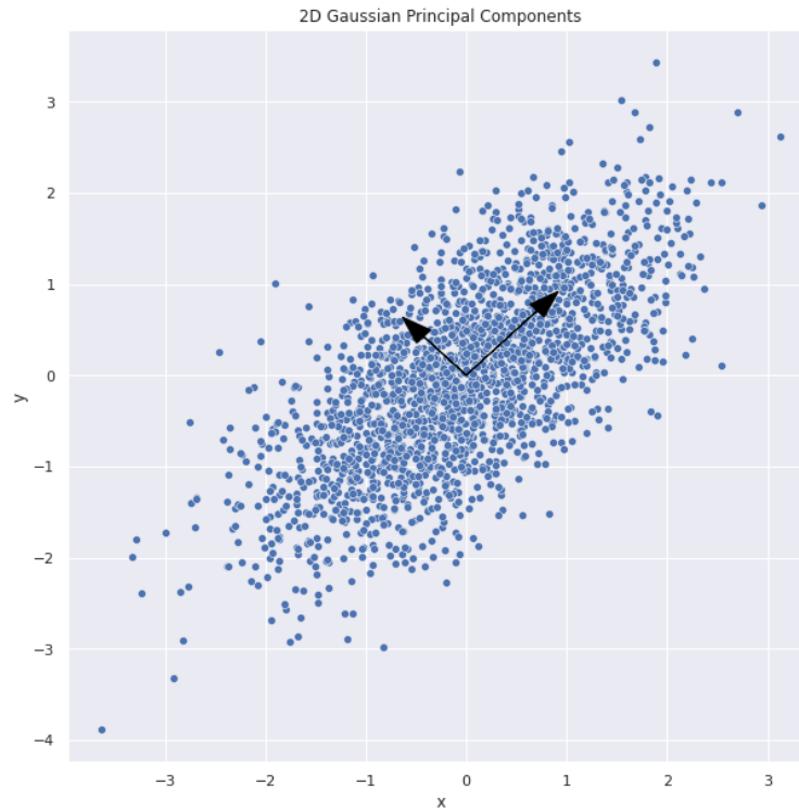
Figure 2.4: Principal components of 2000 points simulated from a 2D multivariate normal distribution with mean at the origin, unit variance and covariance 0.7. The principal component pointing in the top right direction corresponds to the largest eigenvalue and captures the majority of the variability present in the data. The plotted vectors have been scaled for illustrative purposes.
