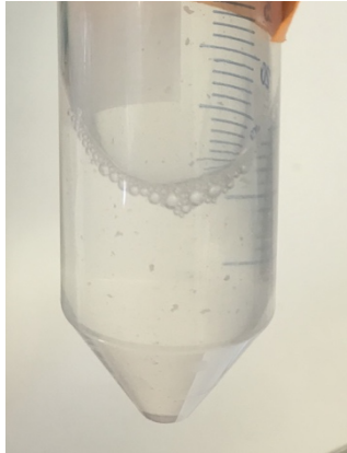
Figure 31: Dried protein powder in Eppendorf tube dissolved in denaturing buffer. Small white particles can be seen floating in the buffer.
