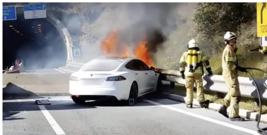
Figure 2: An electric car that has caught fire after an accident [3]
