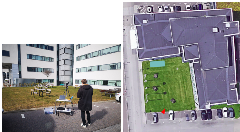
Figure 7.1 Photograph (left) and aerial view (right) of one of the recorded scenes. The red triangle in the right image represents the position and orientation of the radar. The blue rectangle represents the metal container that was missing in the original image.
