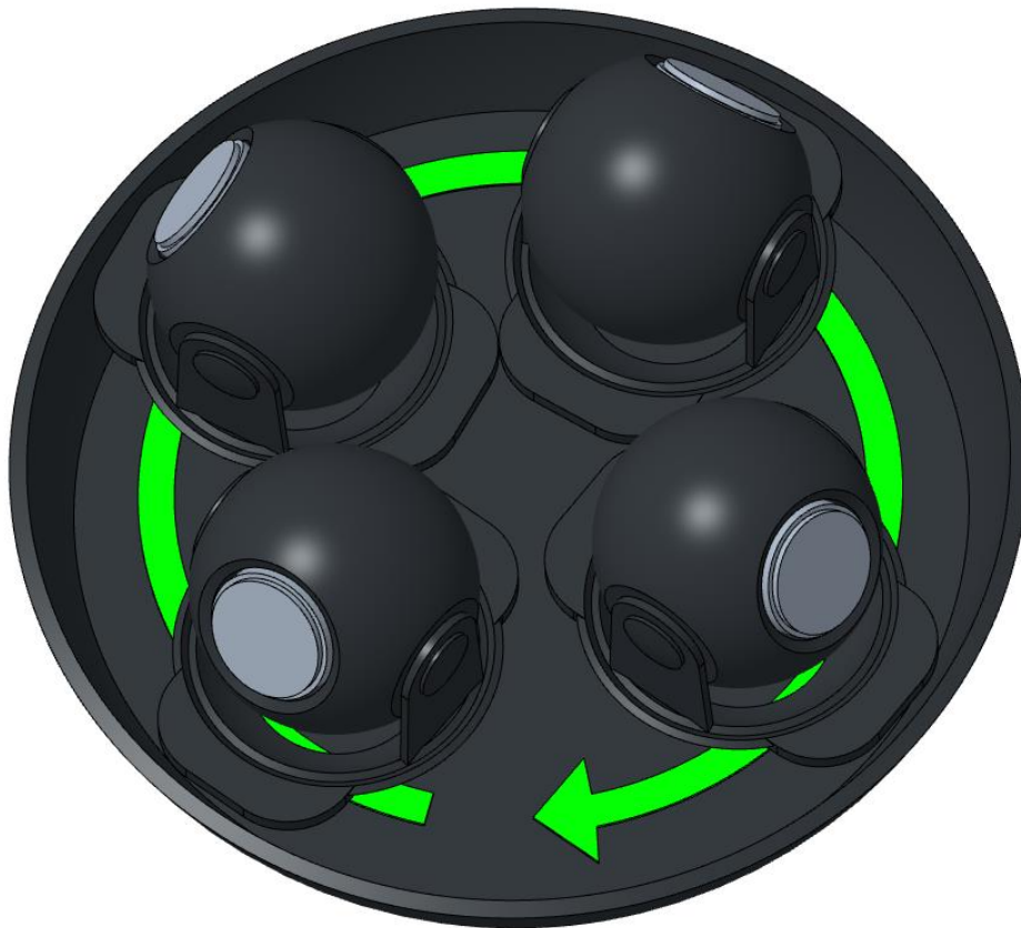
Figure 4: Illustration of the pan movement on the multidirectional camera.
