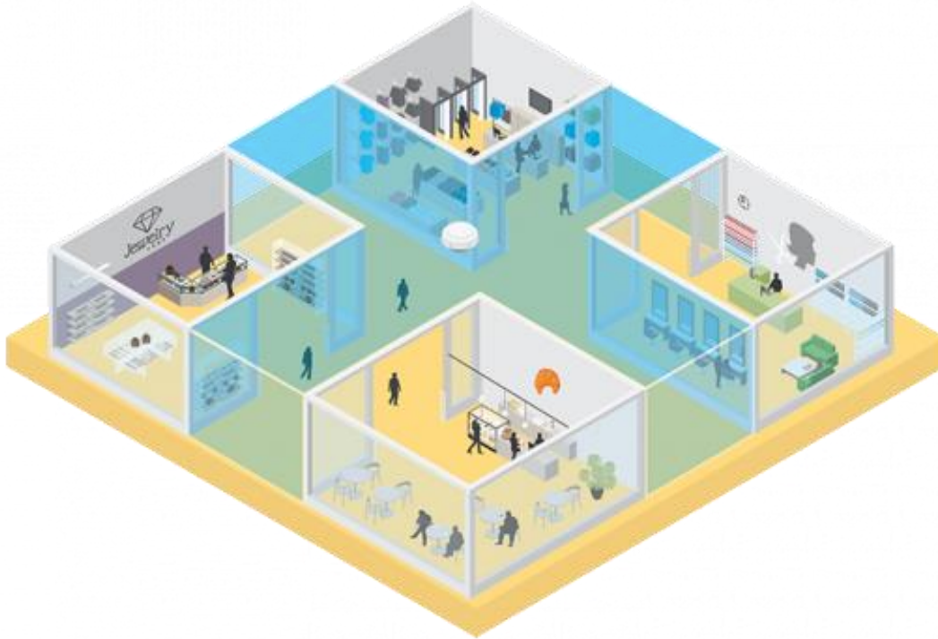
Figure 2: Illustration of the field-of-view of a multidirectional camera. The blue indicates coverage provided by just one multidirectional camera in one of many use cases.
