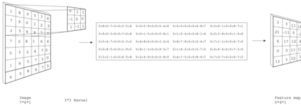
Figure 5: The convolutional stage of a CNN architecture. An input image convolved with a 3 · 3 kernel and filter size 1. The kernel moves across the image matrix, reducing the number of parameters compared to fully connected networks, yielding a 5 · 4 · 1 output matrix.
