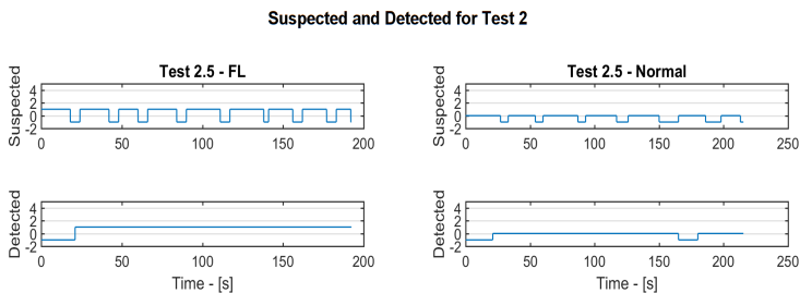
Figure 8.8: Suspected and Detected for Test 2.5 with minispare on FL and normal tyres
