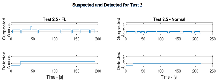
Figure 8.5: Suspected and Detected for Test 2.5 with minispare on FL and normal tyres
