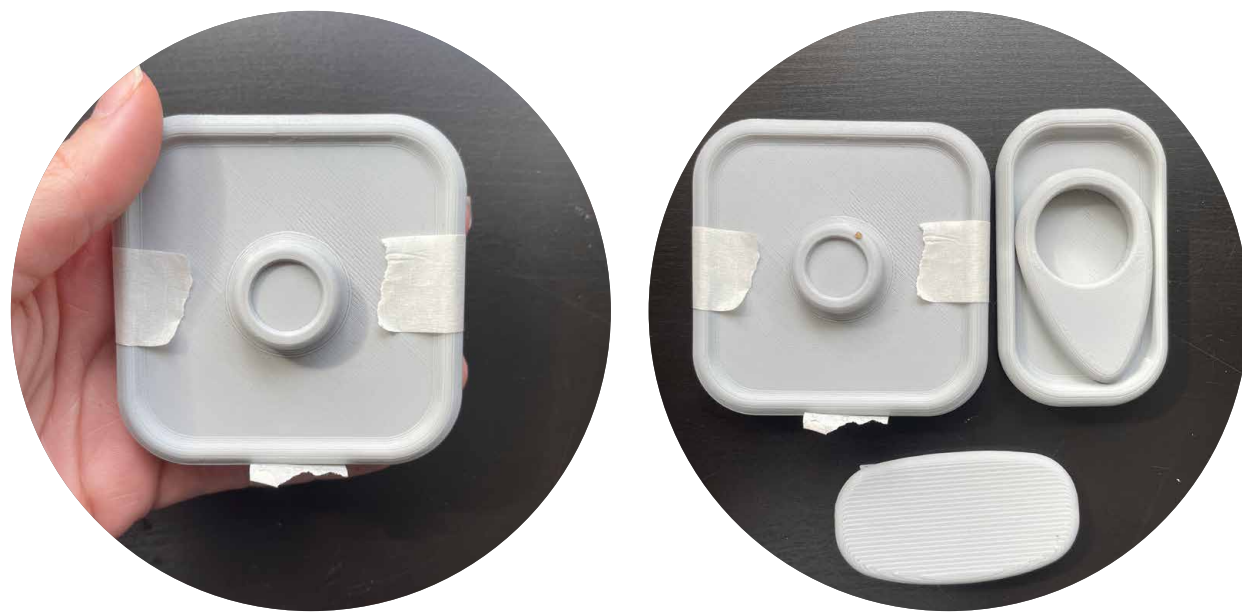
Concept 05, 3-D printed to test usability and dimensions. I realized that dimensions were too small for ergonomic purposes, and for the screen. The gripping part of Concept 05 could be bolder and bigger for holding.
