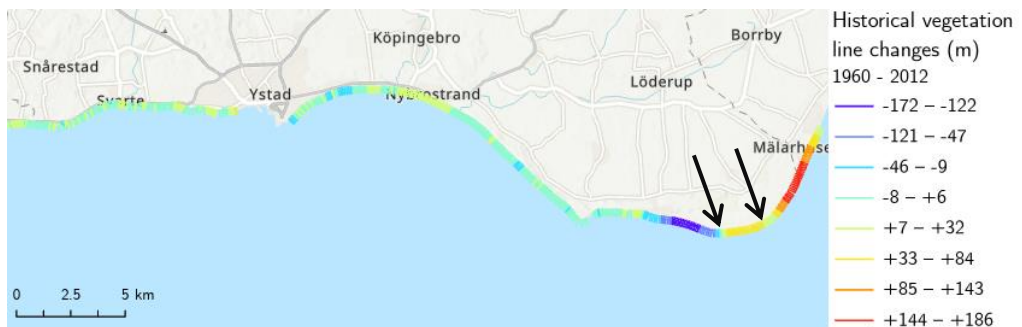
Figure 5.2: Historic shoreline change in Ystad municipality between 1960 – 2012 from Fredriksson et al. (2017). Areas where the Bruun Rule is applicable in its strict form are indicated with black arrows.
