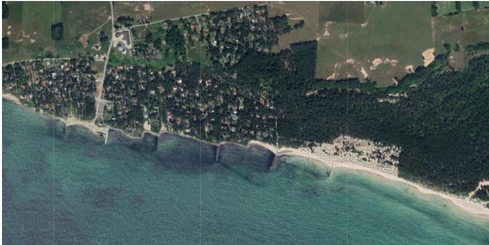
Figure 3.3: Overview of Löderups Strandbad. The rock-reinforced coastline is visible as the section where no beach can be seen. The groynes are seen as the lines perpendicular to the shoreline. Source: Scalgo Live (n.d)
