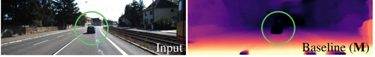
Figure 11: Example of a infinite depth/ "hole" that is caused by moving objects that has the same velocity has the camera. [7]
