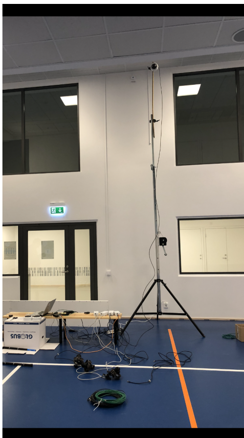
Figure 5.6: Tripod with an extra broom on top to reach the desired height. In this image only the highest camera is mounted.
