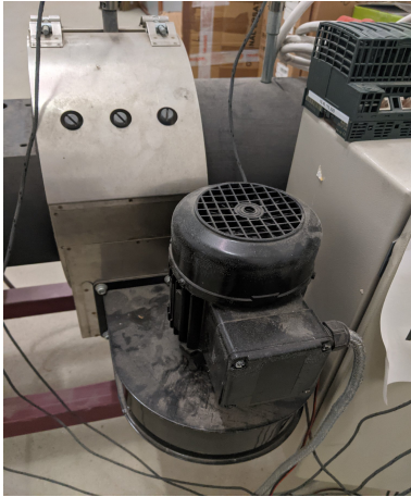
(a) Air cooling fan.
