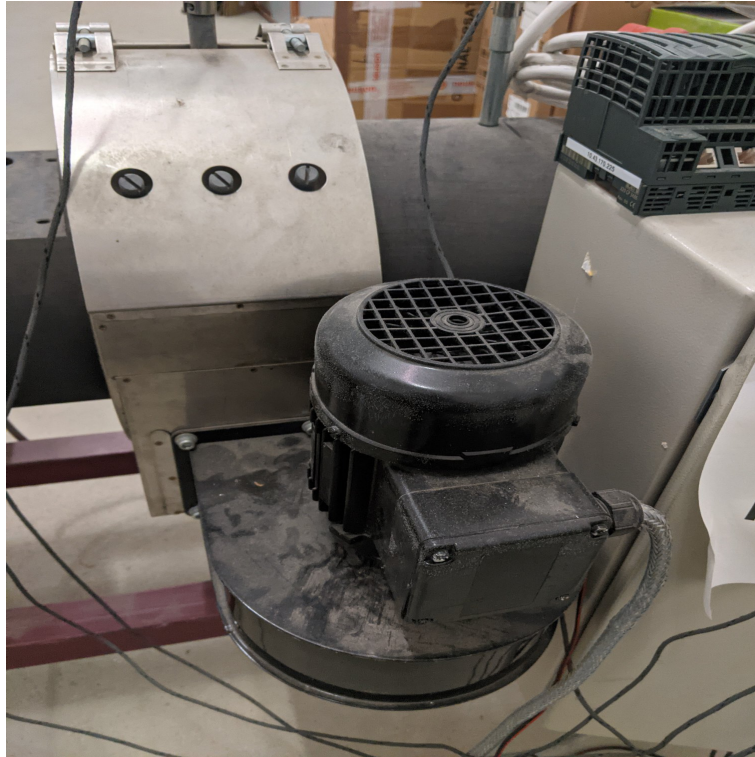
Figure 1. The centrifugal fan used for cooling, which is the main cause of the nonlinear dynamics in the extruder problem considered.
