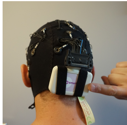
(b) EasyCap EEG cap. The Smarting amplifier is attached to the cap using elastic bands.
