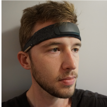
Figure 3.4: The Muse S amplifier attached to the EEG cap. The white strip near the ear is one of the electrodes.
