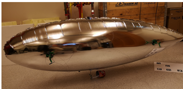
Figure 3.13: Picture of the final blimp with all components attached.
