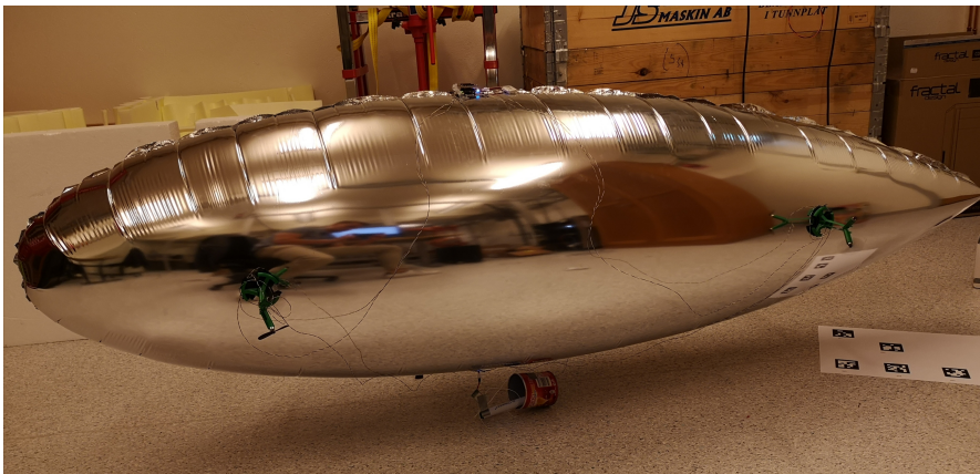
Figure 1.1: Picture of the blimp UAV used to perform real-time experiments.
