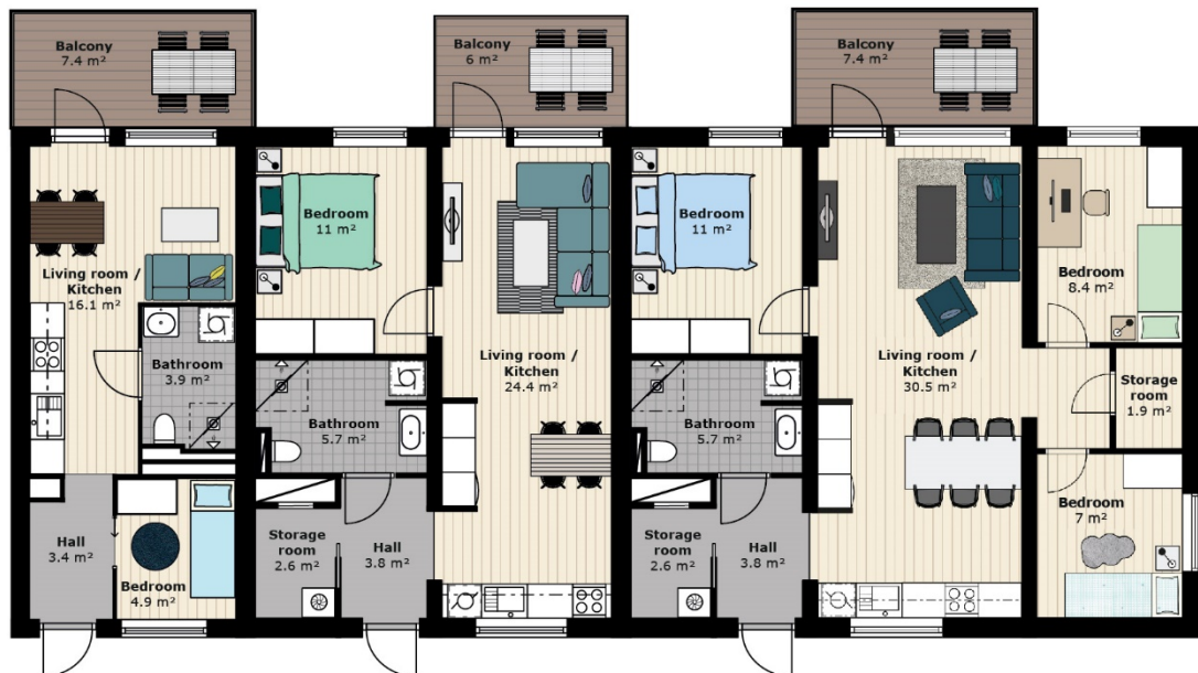
Figure 3.1. Apartment floor plans. From left to right: small two room apartment (2S), large two room apartment (2L), four rooms apartment (4). Image provided by BoKlok Norway.
