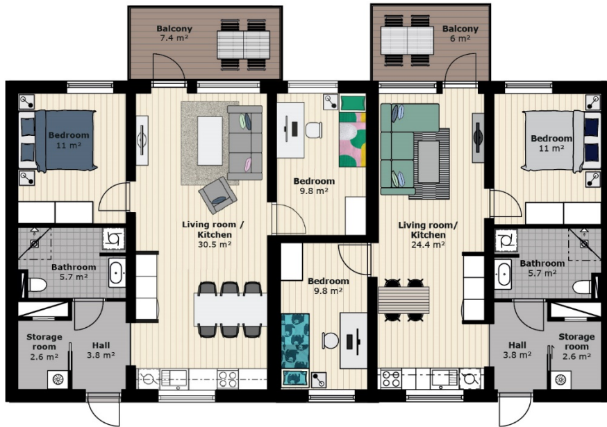
Figure 3.2. Apartment floor plans. Left, large three room apartment (3L). Right, small three room apartment (3S). Two three room apartments must be placed together as they share a module. Image provided by BoKlok Norway.
