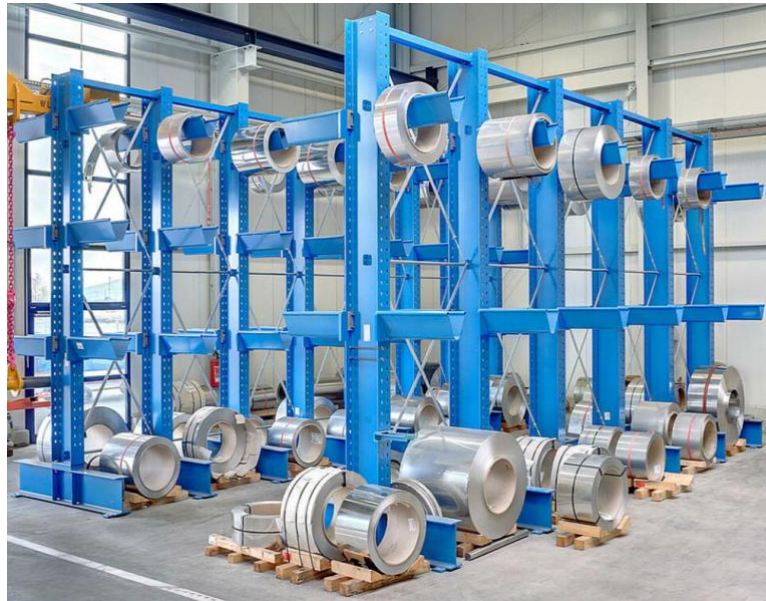
Cantilever rack, (OHRA GmbH, 2021)
