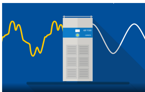
Figure: Illustration of the working principle of an active filter. Filtered signal to the right. Figure from Comsys ABs homepage.
