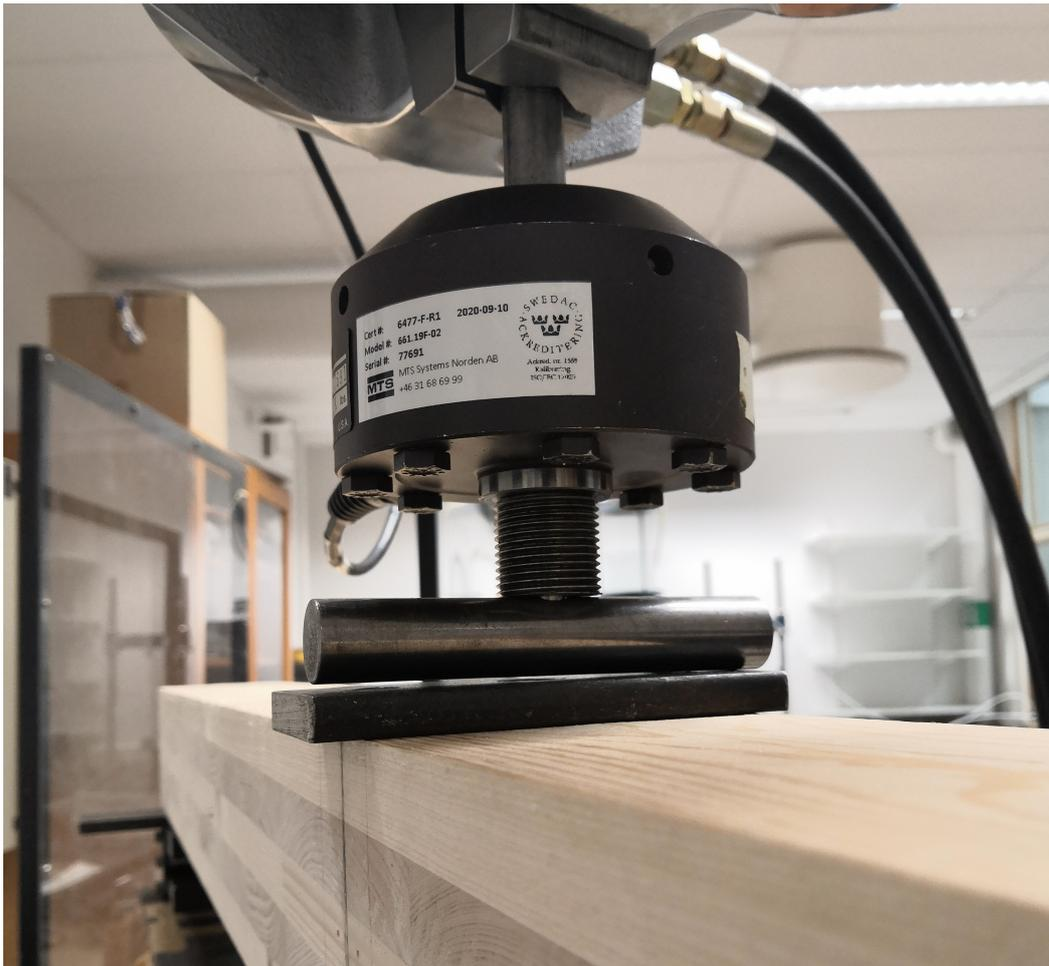
**Figure B.7:** Initial load application conditions due to slope of test rig and CLT-beam, see Figure B.5.
