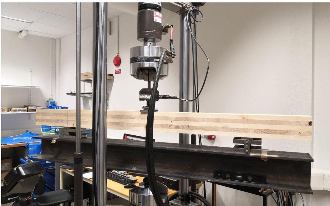
**Figure B.2:** Test setup for out-of-plane loaded Specimen 1 beam.
