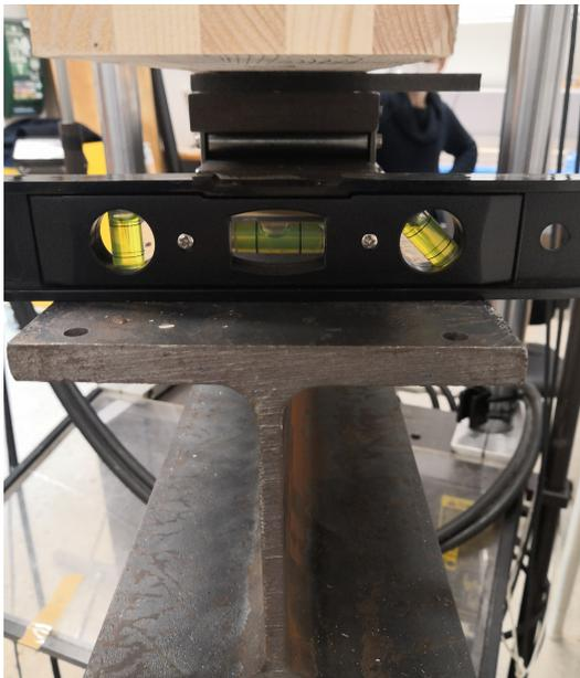
(a) Slope of I-beam test rig.
