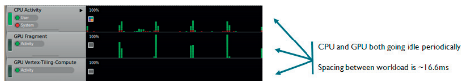
Figure 2.1: Screenshot from Streamline of a GPU and CPU idling each frame when the Dynamic Voltage and Frequency Scaling frequency selected is too high [2]
