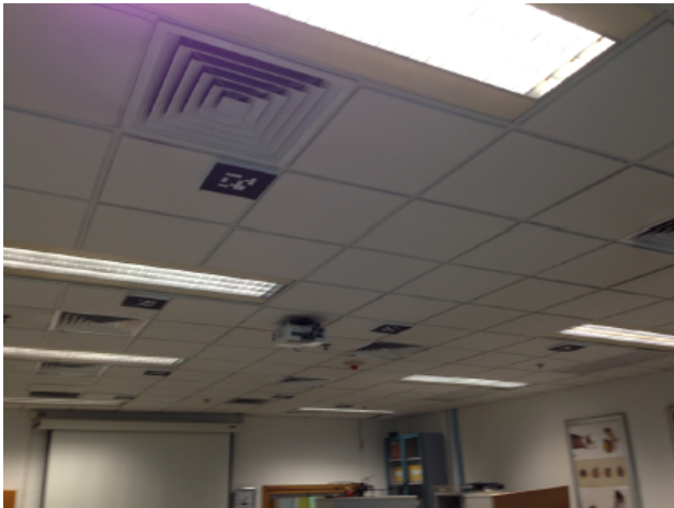
Figure 3.7: Experimental setup for ceiling mounted navigation codes [Dzodzo et al., 2013], © 2013 IEEE.
