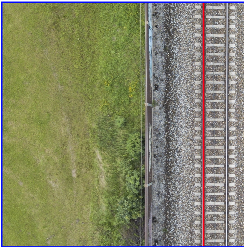
Figur 5.4: The red line is the rail that the Optram measurement while InSAR measures the whole image (Müseler, 2018)
