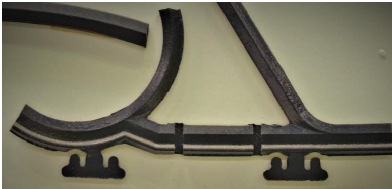
Figure 4.6 Poor surface on the gasket
