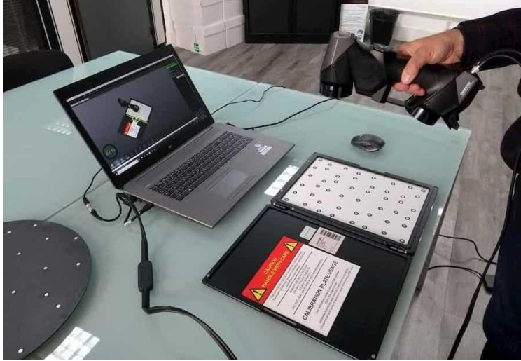
Figure 5.31 Calibration set up [54]
