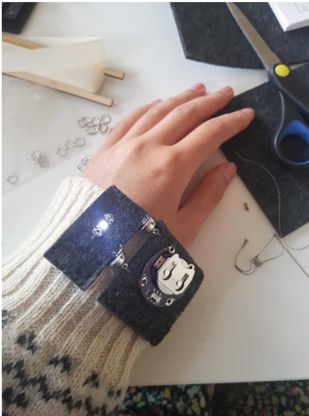
Evolution of magnetic and clip solution. Magnetic clips for attaching on the edges of clothing. Simple securing and removal.
