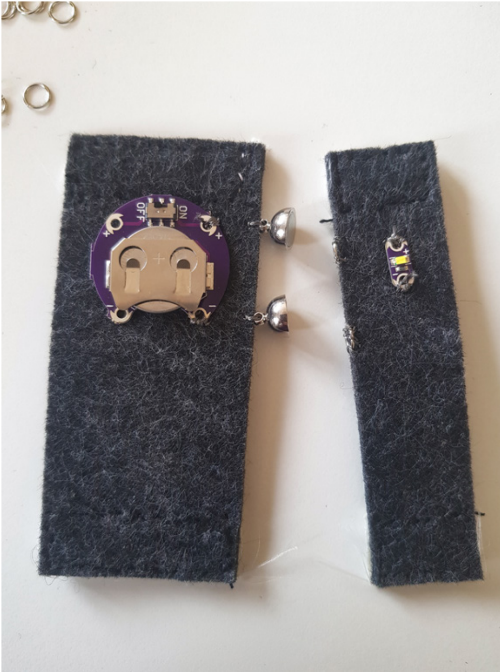
Magnetic connectors on the sides for connecting pieces to one another. Shown above is a battery piece and an LED piece.
