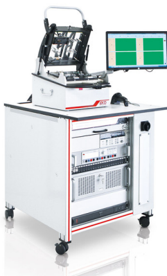
Figure 2.1 Displaying a test fixture with instruments inside a 19 inch rack.
