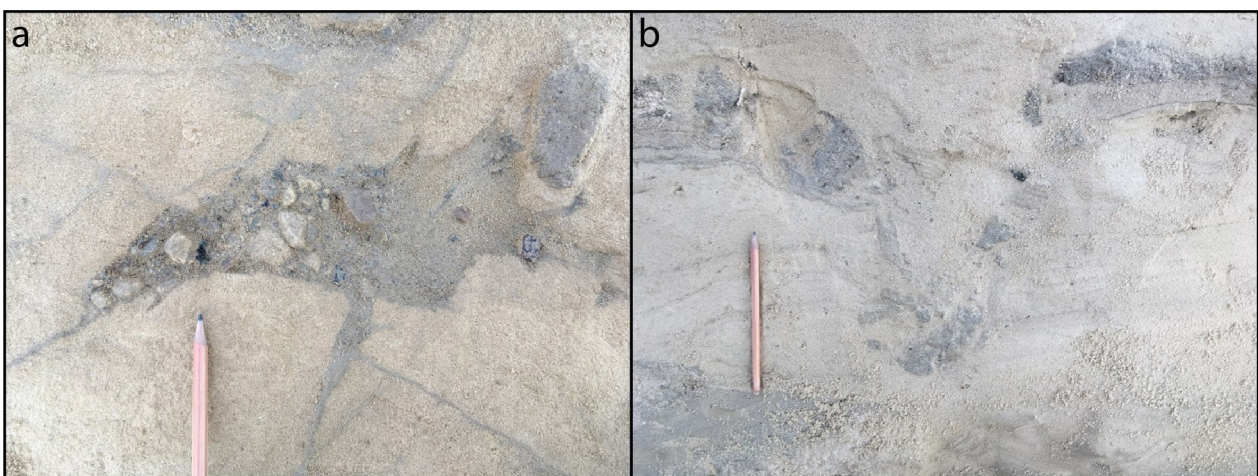
Figure 20: Close up photographs taken within section 3, see pencil for scale. a) Sediment pocket within the limestone in which larger clasts (~2 cm in size) are concentrated in the left half of the pocket, whilst clay-rich sand dominates in the right half. b) Deformed, V-shaped, fragmented horizon of massive, clay-rich fines situated in massive, sorted, lime-rich sand.
