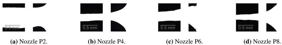
Figure 44: One end of the channel of samples made with different nozzle sizes. a) shows a channel made with nozzle P2, b) shows a channel made with nozzle P4, c) shows a channel made with nozzle P6 and d) shows a channel made with nozzle P8. Note that the "vertical channel" is an artifact of the data collection process rather than any form of side channel.
