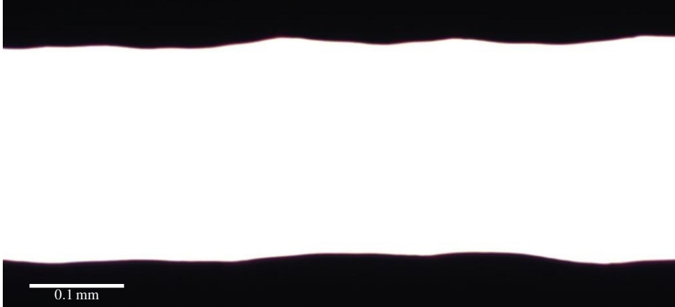
Figure 10: The actual shape of a sub-millifluidic channel made with FDM that was intended to be straight. The channel walls can be seen to have an undulating irregular shape.
