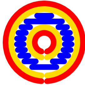
Figure 13: Simple illustration of one layer of a cylinder with a hole in the middle made with FDM. The three basic types of lines of deposited material are shown in different colors. External perimeters are shown in red, internal perimeters are shown in yellow and infill is shown in blue.
