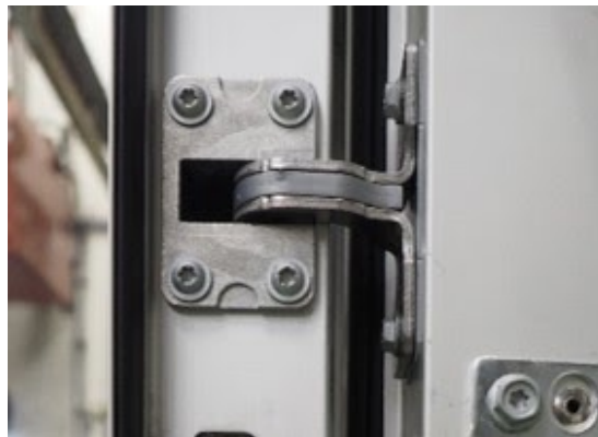
Figure 4.16 - Look of the hidden hinge seen from the space between inner and outer Passdoor frame.
