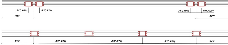
Figure 4.51 - Alternative mounting layout for the hinges along the frame stile.
