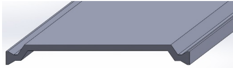
Figure 4.5 - Cross sectional view of the broken cold bridge, specially designed with dimensions to fit the threshold and tube stiles of the OH1082P Passdoor.
