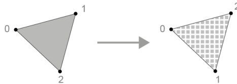
Figure 17: The Orienter transformer in FME changes the orientation of a surface by changing the order of the vertices of polygonal features. Here the back is represented with a checkered pattern for distinction. If these faces were lying horizontally (surface normal), the outward-facing triangle would have a surface normal z -value of 1, while the inward-facing would have -1.
