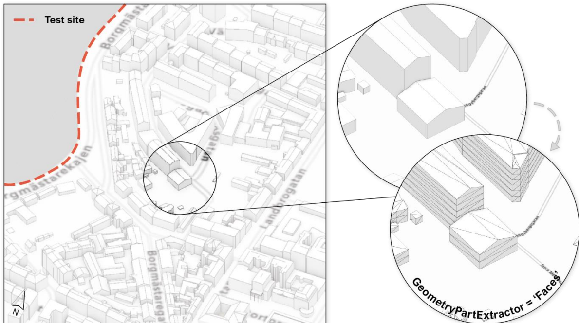
Figure 14: The process of extracting faces from multi-surfaces was applied on the test data, resulting in separate records per each face part of the building models.
