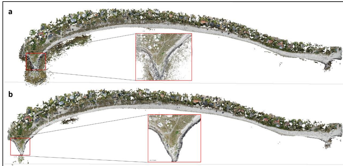
Figure 20 – Difference between sparse point clouds when using the water mask (b) during image alignment and without (a).
