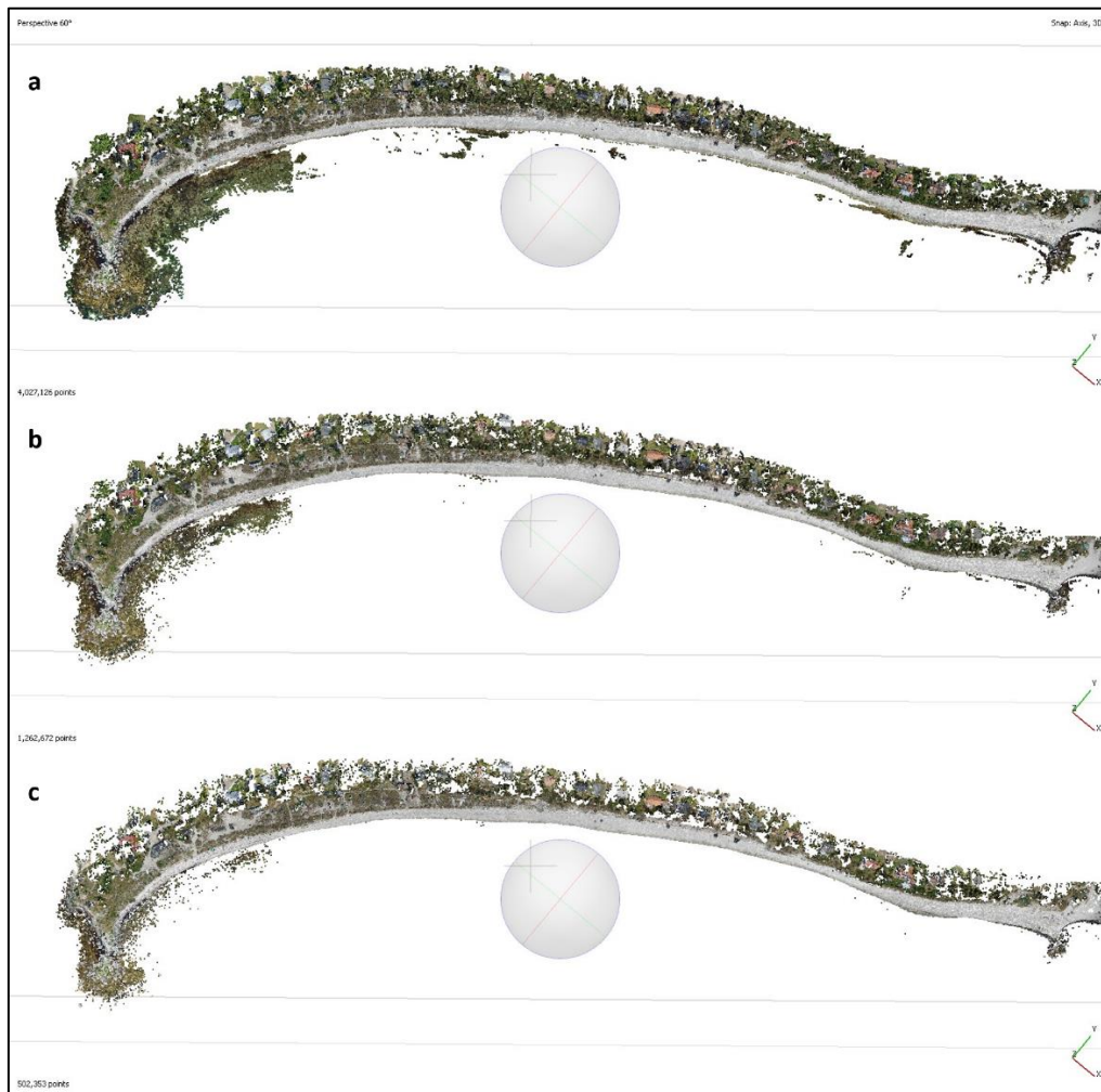
Figure 13 – Visual comparison of three sparse point clouds in Agisoft Metashape. 13a showing a point cloud before any optimization with ~ 4,000,000 tie points. 13b showing the optimized point cloud as derived in this thesis containing ~ 1,200,000 tie points. 13c shows an overly optimized point cloud with many gaps, containing ~ 500,000 tie points.
