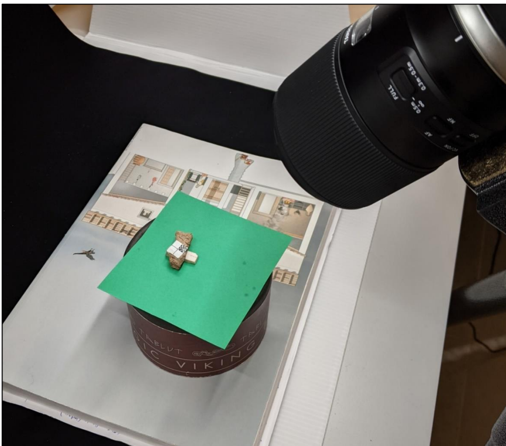
Figure 9. Photograph acquisition set up: digital camera, lightbox, tripod, and improvised stand (lid from a boardgame on top of a book) to provide optimal distance between lens and object. Pictured is the Huseby Klev bear phalange. It was balanced on top of a piece of rubber eraser to provide better acquisition angle. A millimetre-scale (10x10mm) was placed on top of the bone, next to the cut mark.
