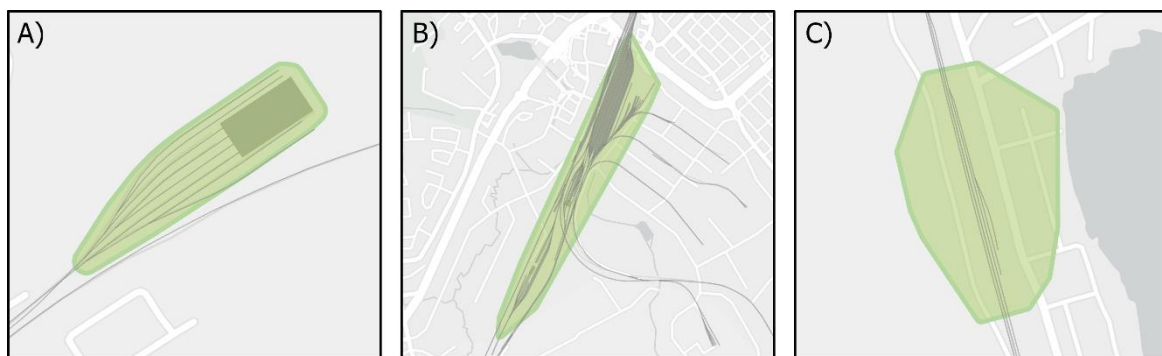
Figure 11: Examples of geofence categories. A) Category A: Geofence separate from main rail network. B) Category B: Geofence at freight yard. C) Category C: Geofence close to main rails. Sources: Esri, HERE, Garmin, Lantmäteriet, USGS, OpenStreetMap.
