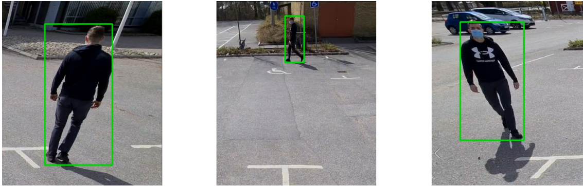
Figure 5.3: Three different images with bounding boxes detected by YOLOv4 applied to it.
