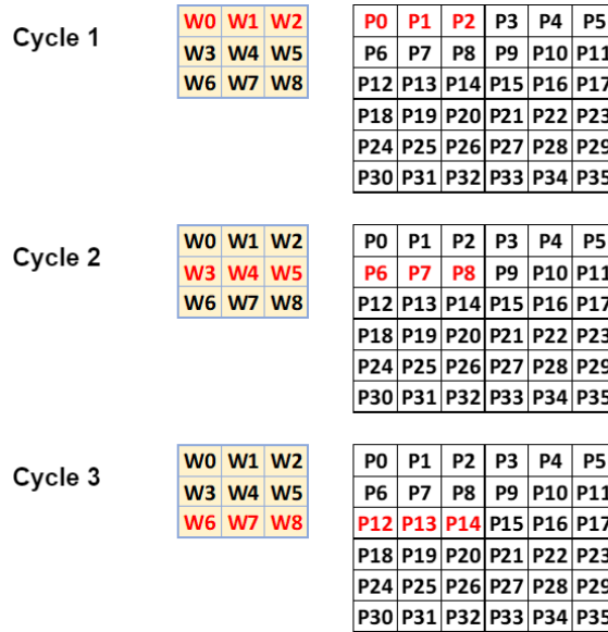
Figure 3.5: Visualization of weights and pixels used in each cycle to compute one output pixel during convolution.
