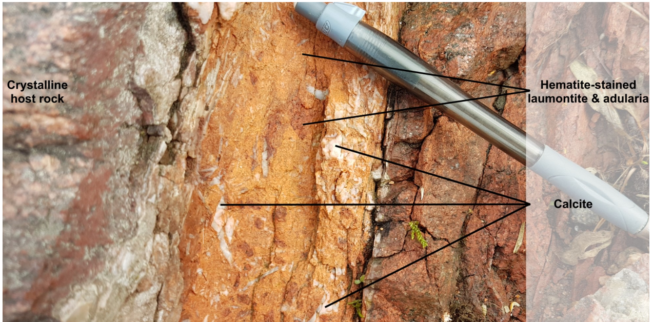
Fig. 5.8. ABR200014: Detail of border of main brittle deformation zone oriented 265/85. The light orange and darker red fine-grained fault core consists mostly of hematite-stained laumontite and adularia. The milky white grains are calcite aggregates.
