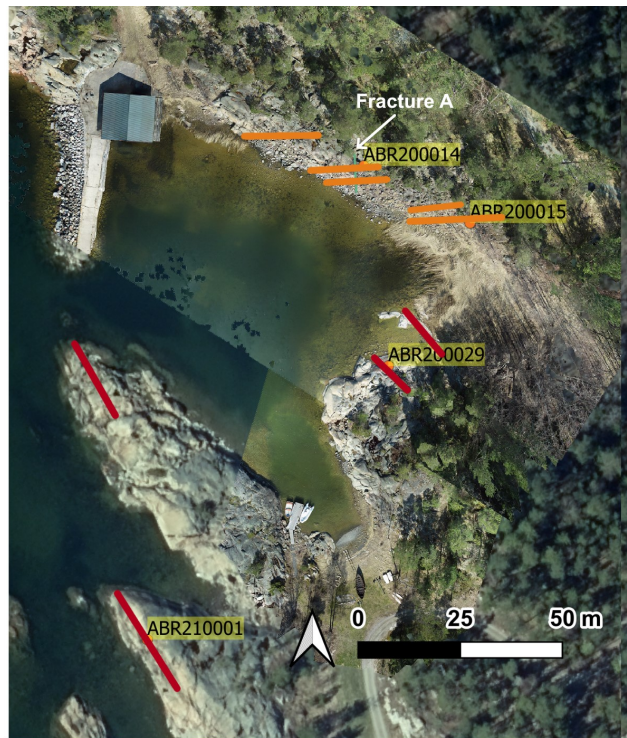
Fig. 4.11. Brittle deformation zones at localities (from N to S) ABR200014, ABR200015, ABR200029 & ABR210001. Kinematics interpreted from slickensides.
