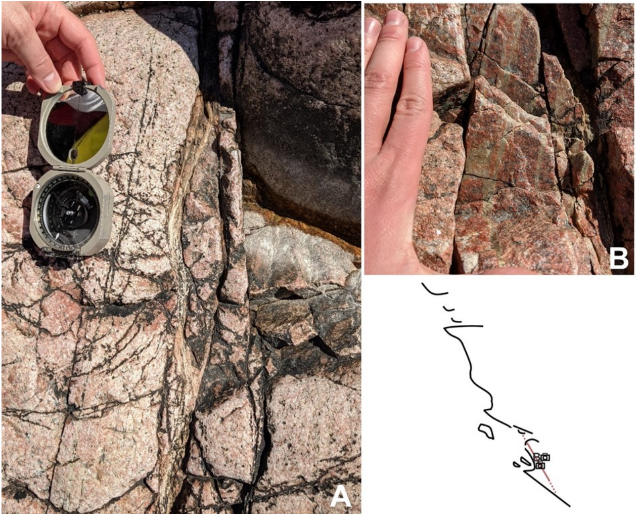
Fig. 4.9. A. ABR210003: Top-down view of a band showing grain size reduction (mylonitisation) cut by the 0.5 meter-wide fracture set. B. ABR210003: Vertically dipping sealed fracture network striking 150.
