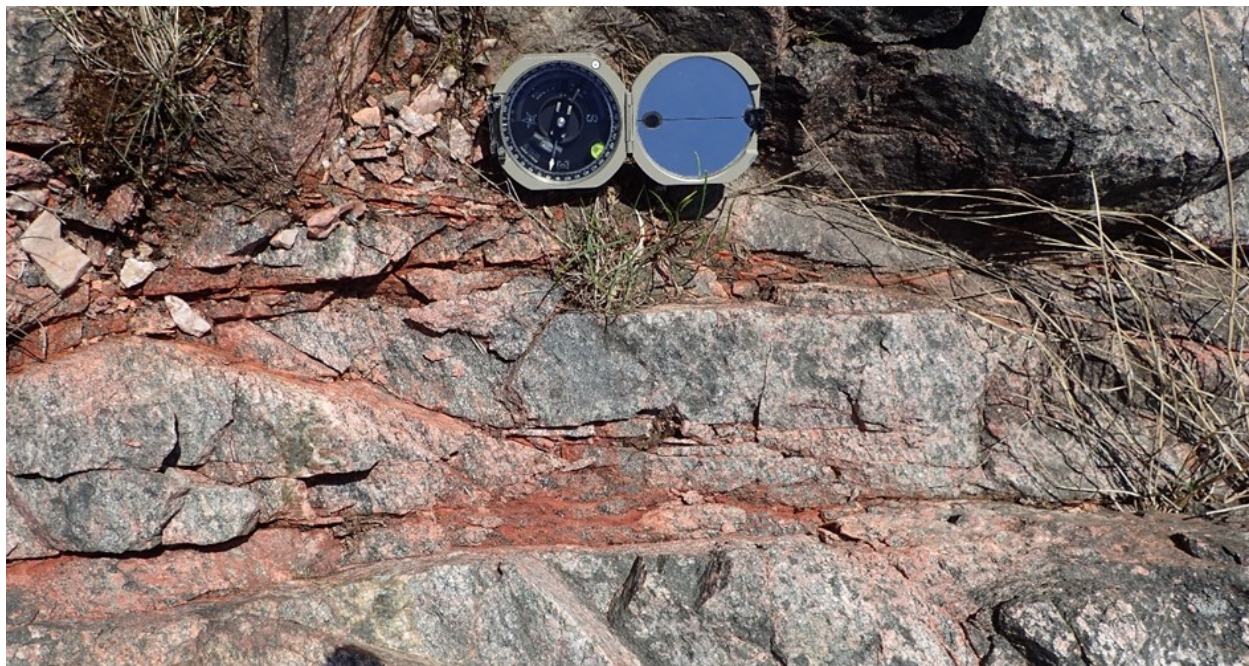
Fig. 4.17. ABR210010: E-W striking steeply dipping red-stained fractures. The fracture minerals have a greatly reduced grain size compared to the crystalline host rock.
