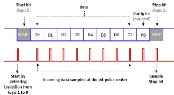
Figure A.1: Break down of UART transmission. Courtesy: Soliton Technologies[12]
