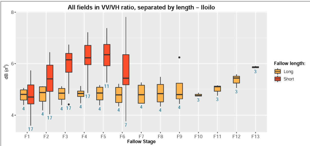
Figure 10. Boxplots of the backscatter coefficients for fallow separated by fallow duration (short and long) in Iloilo for VH (top), VV (middle) and VV/VH ratio (bottom). Fallow number relates to Sentinel-1A revisit time since the start of fallow.
