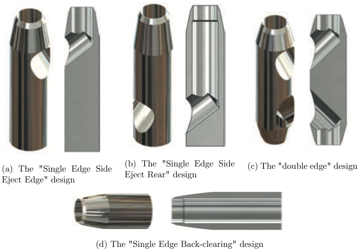
Figure C.1: The four designs in this figure should be possible to manufacture in the transfer machine.
