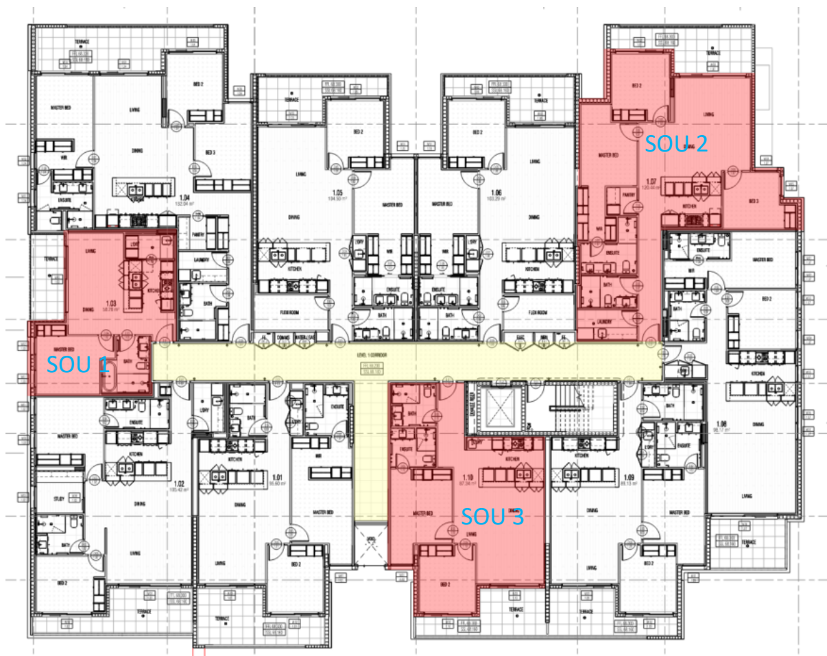
Figure 24: Modelled corridor and apartments on floor Level 1.
