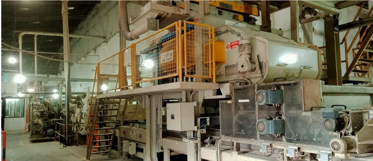
Figure 22: Interconnected UPVC Board Cutting Machines (Company 'J' Factory Premises)
