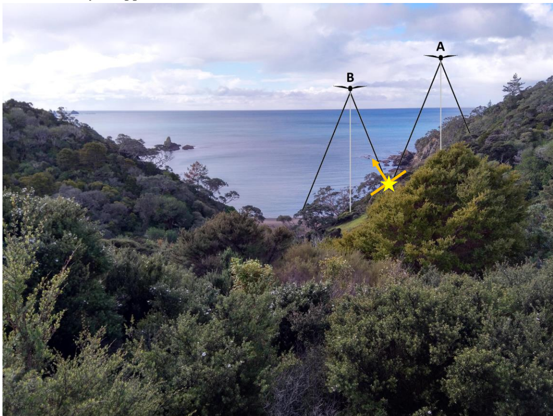
Figure 3: Scanning geometry. Figure demonstrates how incidence angle is a product of scanning angle and terrain slope. Surveyed point (yellow star) is positioned between the flight path centres of A and B. Because of the terrain slope, incidence angle for B is close to 90^\circ , while the incidence angle for A is obtuse, far from normal.
