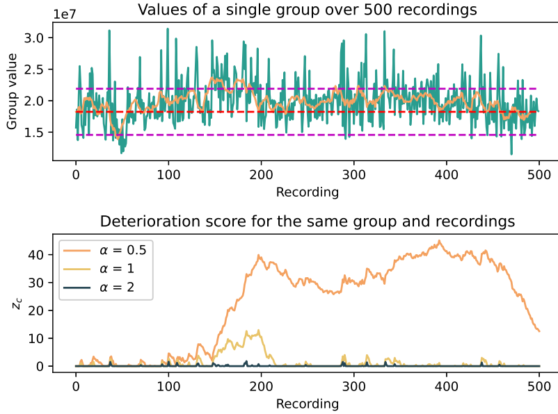
Figure 10: Visualisation of how z_c develops over 500 recordings for one group. The top plot shows the group values of one specific group together with a mean \mu (red dashed line) and one standard deviation \sigma (magenta dashed line) calculated from the first 10 recordings. A 10 point moving average is also displayed in yellow. The bottom plot shows how z_c changes over the recordings with varying \alpha .
