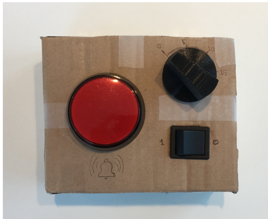
Figure 6.10: The first prototype of the control station.
