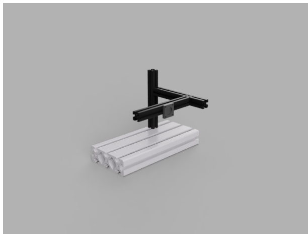
Figure 26: Preliminary blueprint of the item © profile assembled support & positioning system. The base was altered during installation in the chamber during the actual experiment to make removing and putting the support back inside easier and safer.
