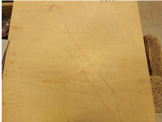
Figure 3.6: The full scale drawing used to make the patterns.
