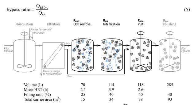
Figure 3.1.Pilot process diagram and reactor parameters. 9 denotes reactors with biomass carriers. 0 denotes aeration. \* Sludge fermentation not operational during exp. period.
