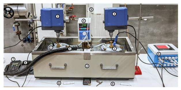
Figure 3.3: Experimental setup with the following components: reactors (1) submerged in a water-bath (2) and stirred with stirrers (3). Heating and cooling units (4, 5). Combined pH and temperature meters (6) and DO meter (7). Syringes (8) and  $N_2$  supply (9).
