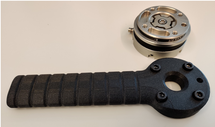
Figure 5.2 Optoforce HEX-E v1 F/T sensor and handle used.
