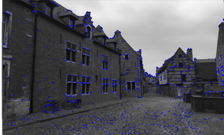
Figure 3.2: FAST detection after optimisation
