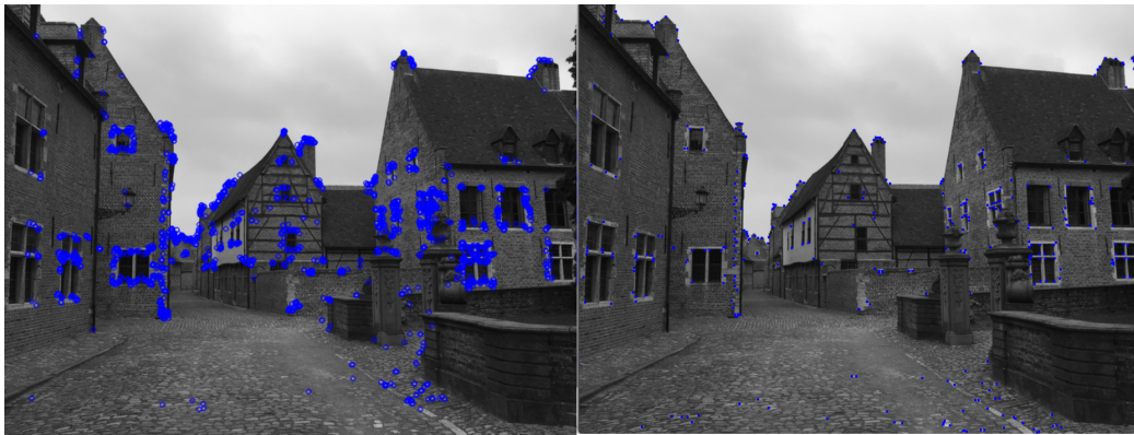
Figure 4.2: Software OpenCV ORB result (Left) compared to Vivado ORB result (Right)
