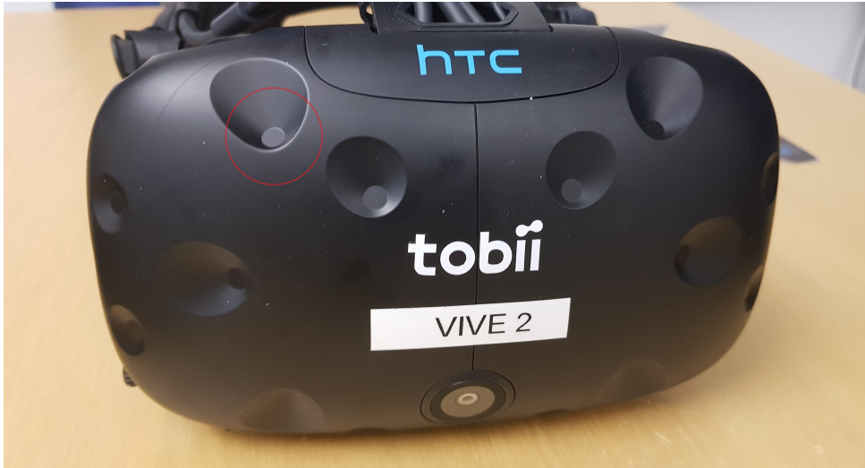
Figure 7: Image of Tobii HTC Vive with one out of several light sensitive photosensors marked with a red circle.
