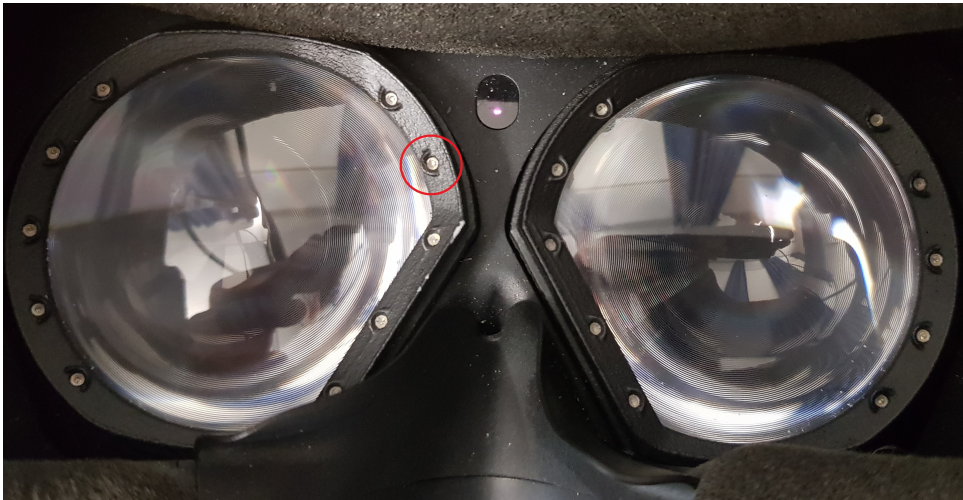
Figure 12: IR Lights in headset, 1 out of 20 illuminators marked with a red circle.
